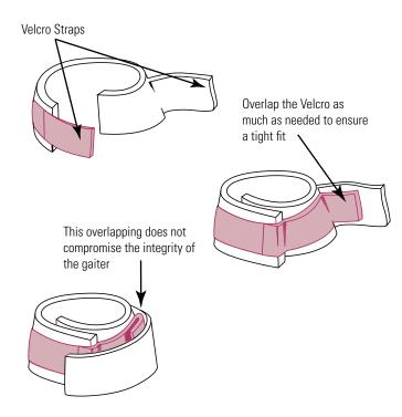
When properly tightened, it should be difficult to fit a finger between the pastern and the top of the gaiter.
