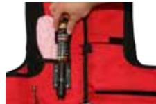
**A** Position of the trigger after the activation: the ball is out of its set, the piston has slid towards the canister and the spring is visible.
