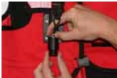
**G** While ensuring that the ball bearing remains in its set, begin to tighten the tap manually. Make sure the ring around the ball bearing is inserted into the recess of the silver piston and is flush.
